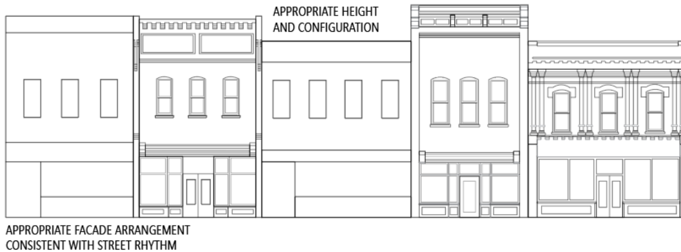
Figure 4: Diagram showing the effect of inappropriate infill. The infill in the upper streetscape is inappropriate in height, scale, and style, and disrupts the rhythm and unity of the block.
