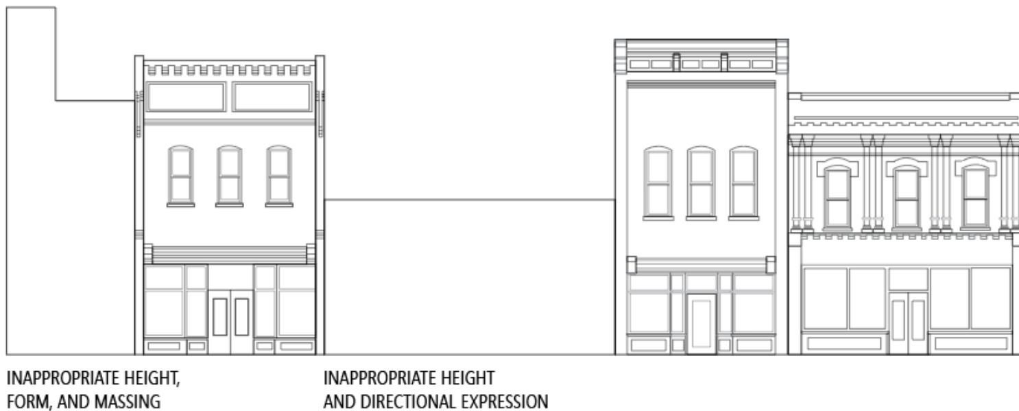
Figure 15: Diagram of inappropriate infill buildings. New construction within the district should be compatible with the height, form, massing, and other aspects of the existing buildings within the district.
